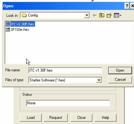
Open the proper file depending on your receiver. All “iTC” hex files are for the StarFire iTC receivers and all “SF” hex files are for older StarFire receivers. Make sure that your receiver is connected to the computer and communicating with the configurator program, then click on the “Load” button to start loading software to your receiver.
