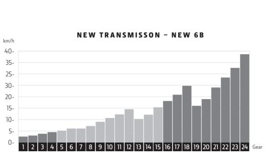
24 gears to fulfil the highest customer requirements and run in every application at the optimum working speed and optimum engine rpm.
