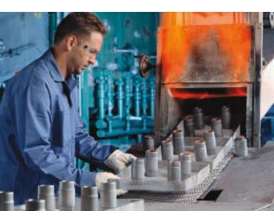
In a patented process, alloy powders, atmospherics, and 2,000-deg. heat fuse the SC-2 coating fast to the part.
