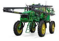
M4040 Rated Hp: 275hp Solution Capacity: 4000L Boom Length: 30.5 - 36.6m Crops Clearance: 170cm Spray Speed: 0-40km/h
