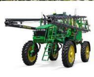
M4030 Rated Hp: 183hp Solution Capacity: 3000L Boom Length: 27.4 - 36.6m Crops Clearance: 170cm Spray Speed: 0-30km/h
