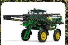
M4025 Rated Hp: 149hp Solution Capacity: 2500L Boom Length: 27.4 - 36.6m Crops Clearance: 160cm Spray Speed: 0-25km/h
