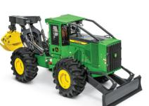
Gross Power: 196 kW Gross Torque: 1,141 Nm Max Grapple Capacity: 1.77 m<sup>2</sup> Operating Weight: 19,713 kg
