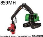
Engine Peak Power: 246 kW (330 h Max Boom Reach: 9.91 m Tractive Effort: 373 kN Swing Torque: 94,740 Nm Tail Swing: 1.94 m - 2.25 m
