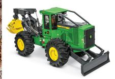
Gross Power: 157 kW Gross Torque: 979 Nm Max Grapple Capacity: 1.77 m<sup>2</sup> Operating Weight: 19,713 kg
