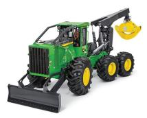
Gross Power: 210 kW Gross Torque: 1,276 Nm Max Grapple Capacity: 2.07 m<sup>2</sup> Operating Weight: 23,697 kg
