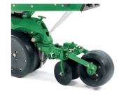
**Disk Closing System** Best for planting at shallow depths in lighter soils. This pushes soil against and over the seed while the press wheel applies pressure for good seedto-soil contact.
