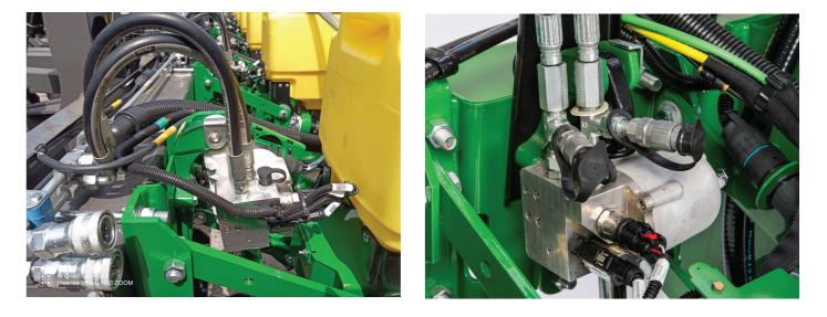
Individual Row Hydraulic Downforce helps ensure consistent planting depth and optimal seed-to-soil contact, even in rapidly changing field conditions. IRHD adjusts downforce up to 5 times per second and can make a 50 kg adjustment in less than 1 second ... Nearly 40% faster than other manufacturers' systems<sup>3</sup>. Our built-in accumulator helps take the shock out of the row unit and assists with your planter's overall ride.
