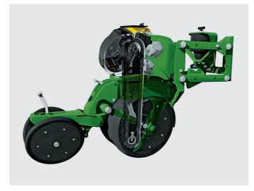
The industry-leading ExactEmerge Row Units is designed to do one thing; put seed into the ground at speed with pinpoint population and spacing accuracy. The key is the exclusive BrushBelt delivery system. The BrushBelt system does not drop seed; it places each seed precisely at the bottom of the furrow with no bouncing or rolling that might affect seed spacing.
