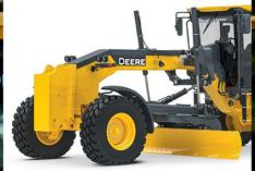
Base Power (1st Gear): 149 kW max traveling speed of 4.0 km/h Max Power (8th Gear): 190 kW max traveling speed of 45.5 km/h Net Peak Torque: 1288 Nm Torque Rise: 55%
