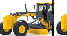
Base Power (1st Gear): 112 kW max traveling speed of 4.0 km/h Max Power (8th Gear): 160 kW max traveling speed of 45.5 km/h
