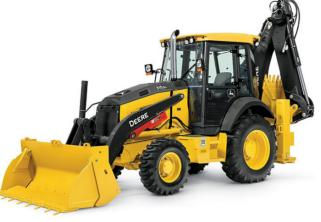
Net Peak Power: 77 kW at 1600 rpm Max. Standard Dipperstick Digging Depth: 3.6 m Operating Weight: 7962 kg Bucket Options: Heavy Duty 0.77 m<sup>3</sup>, 0,8m<sup>3</sup>, Heavy Duty Long Tip 0,96 m<sup>3</sup> & Multipurpose 0.96 m<sup>3</sup> Backhoe Specifications: 610-mm x 0.28-m<sup>3</sup> bucket
