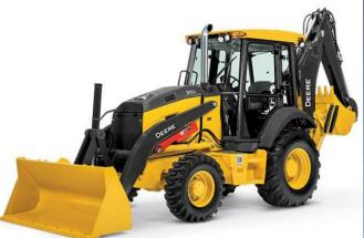
Net Power: 62 kW at 2000 rpm Max. Standard Dipperstick Digging Depth: 3.9 m Operating Weight: 6898 kg Bucket Options: Heavy Duty & Multipurpose 1 m<sup>3</sup> Backhoe Specifications: 610-mm x 0.21-m<sup>3</sup> bucket
