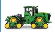
**9RX Engine Type**: JD14 (13.5L), 6 Cylinder, Turbocharged Diesel **Rated Hp:** 490hp - 640hp **Maximum Hp:** 539hp - 691hp **Transmission:** PowerShift /E18<sup>™</sup> **Base Machine Weight:** 24 640kg - 30 390kg **Hydraulic Capacity:** 208 L/Min - 416 L/Min
