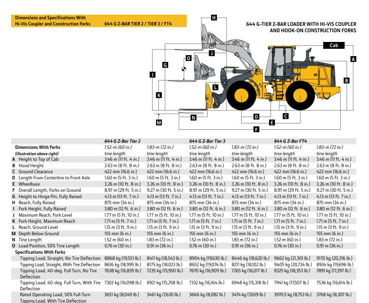
\*Rated operating capacity based on Deere attachments only. 644 G Z-BAR TIER 2 Adjustments to Operating Weights and Tipping Loads With Buckets
