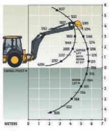
Lift capacities are over end with stabilizers down and tires tangent to ground.
