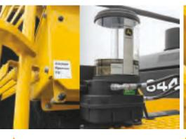
Pump and reservoir include a remote line for ground-level reservoir fill. System features an inlet filter before the pump with both a low-level sensor and an empty reservoir switch.
