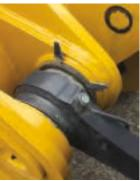
Unlike many aftermarket systems comprised of complex hose connections, the Deere auto-lube option includes hard lines with mounting locations and line routings designed into the machine structure.
