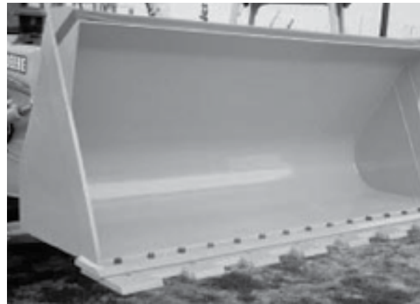
Backhoe loader bucket equipped with T825330 (1-in. x 6-in. x 11 7 / 8 -in., 5/8-in. bolts) short standard sections, and T825333 and T825334 end sections.
